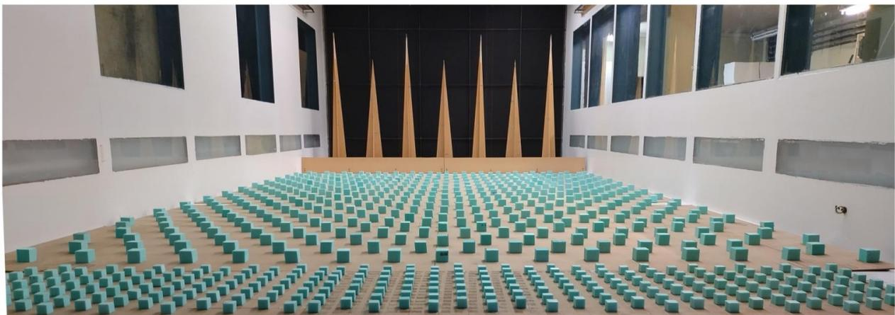
Figure 19 Set up of the fetch of the atmospheric boundary layer (ABL) upstream of the turntable at NTUA
