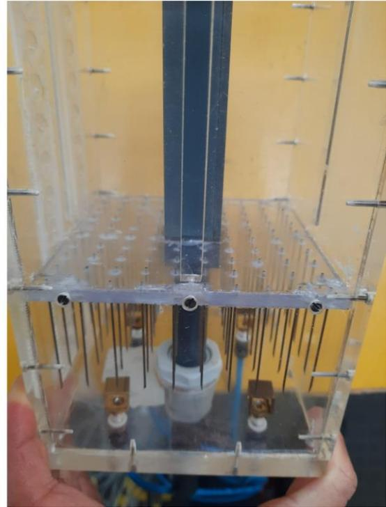
Figure 4 Ceramic heating elements and area source in cube bottom with hypodermic needles and plenum chamber.
