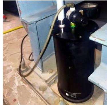
Figure 8 Droplet generator (TSI model 9307)
