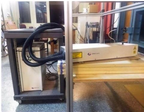
Figure 9 Laser apparatus (LYTRON 200 mj Nd:YAG)
