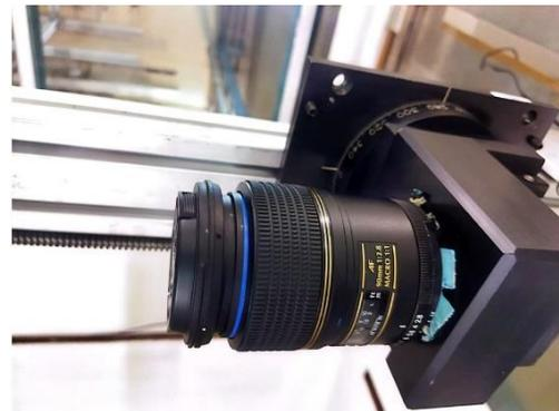
Figure 10 High-speed PIV camera (TSI PowerViewPlus 4MP)
