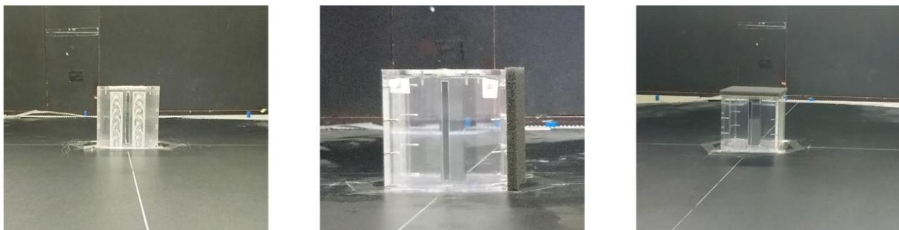
*Figure 1* Cube shaped building with vertical openings in boundary layer wind tunnel. Left: cube without vegetation (bare); Middle cube with façade greening at the windward wall; Right: cube with roof greening.
