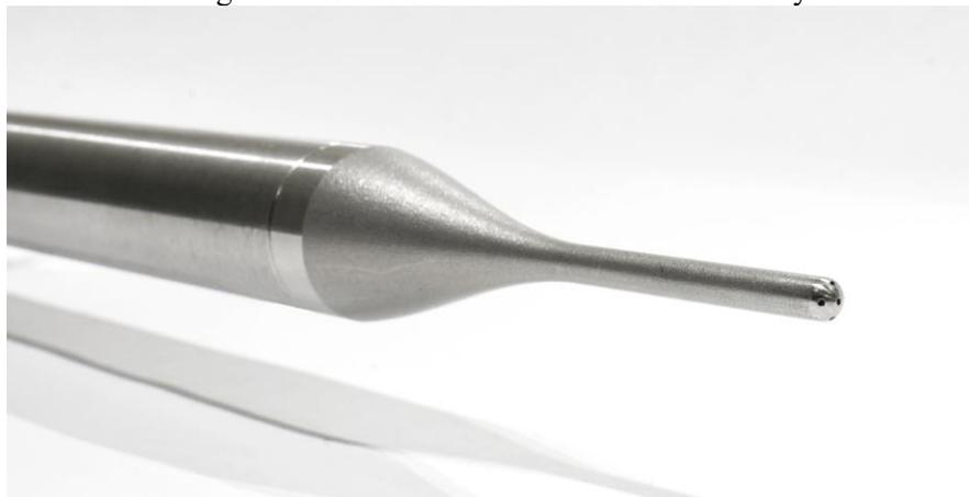
**Figure 3.** Fast-response five-hole probe equipped with piezo-resistive sensors, adapted from [2].
