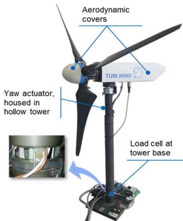
**Figure 4.** The G1 wind turbine with highlighted components
