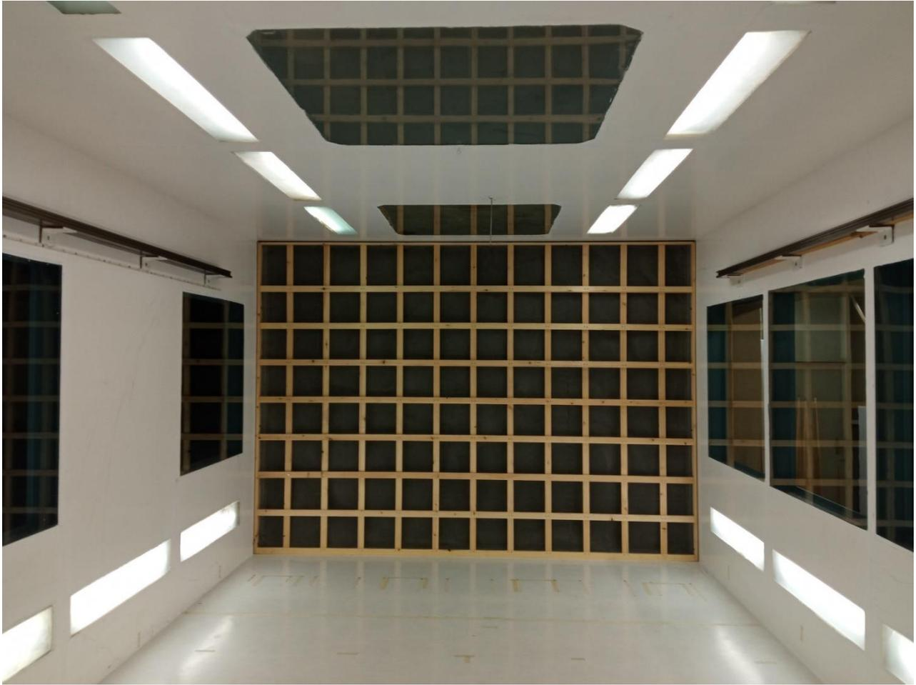
**Figure 14.** Upstream view of the test section with the passive grid installed.
