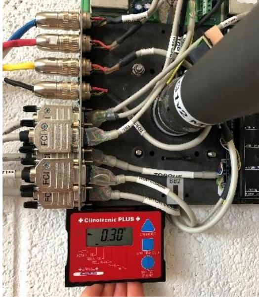
**Figure 12.** Position of inclinometer for tower calibration
