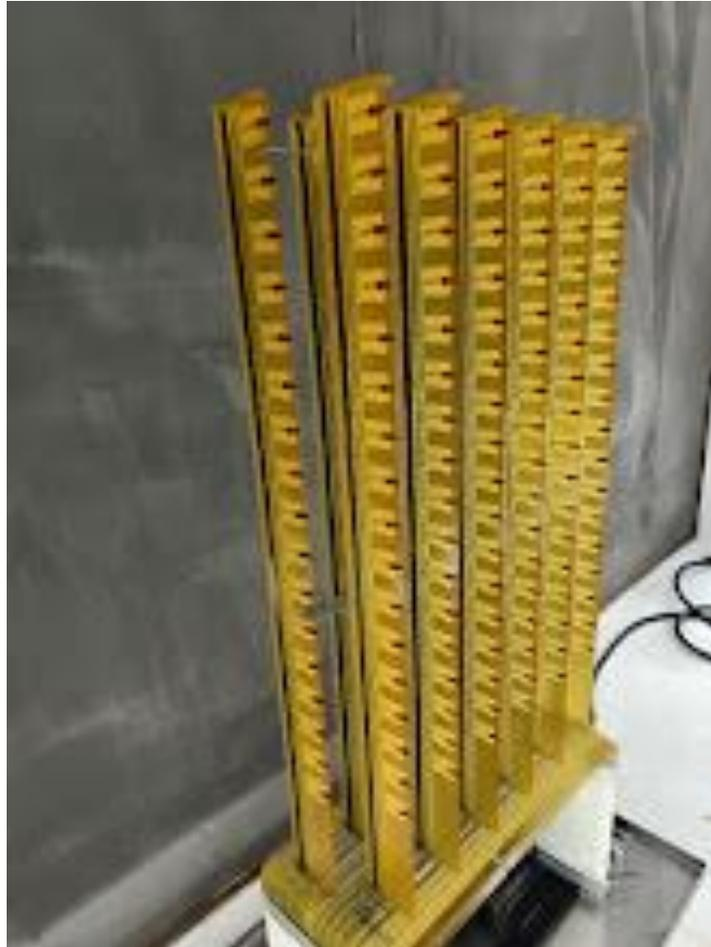
Figure 20. Seeding rake in the wind tunnel test section
