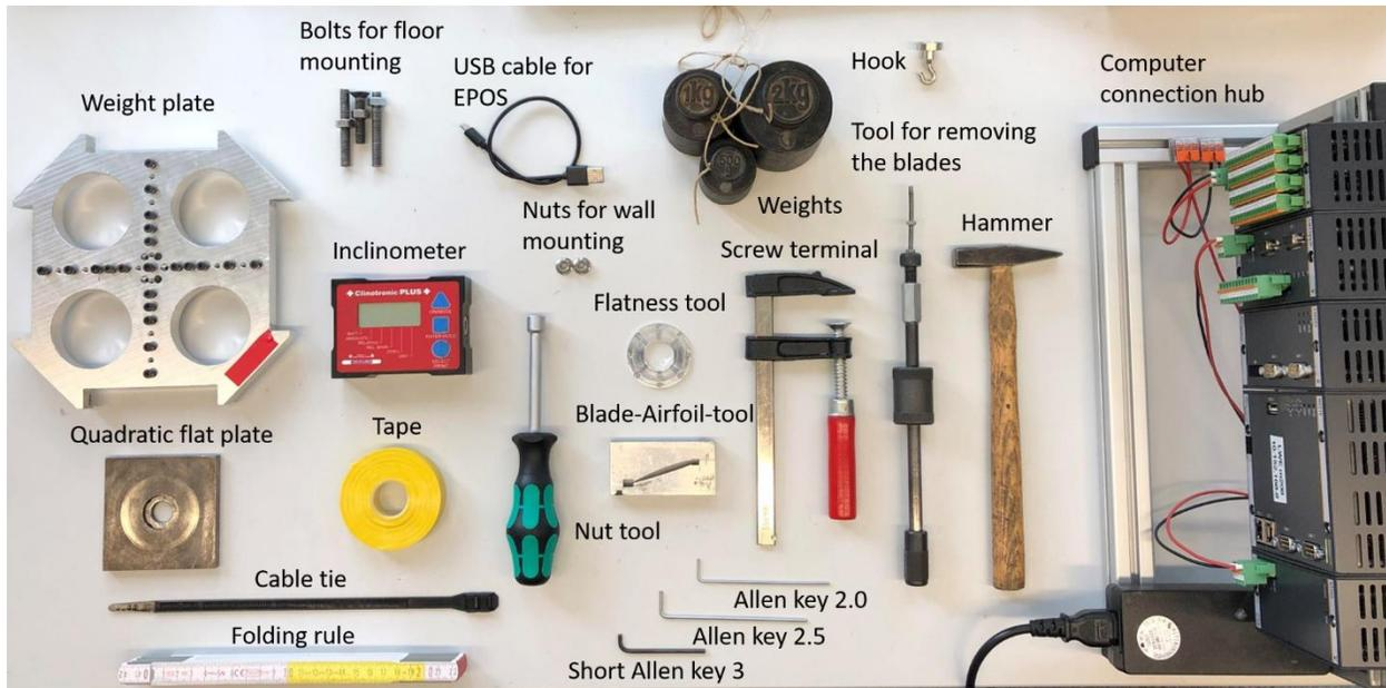
**Figure 7.** Tools needed for calibration
