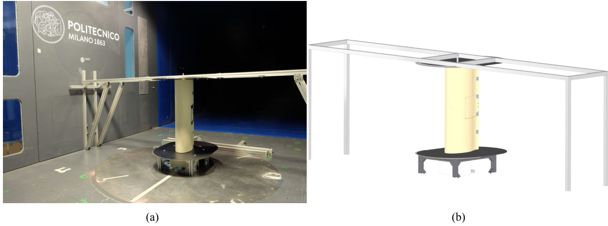
Figure 5: (a) View of the installed model at the GVPM. (b) CAD Assembly of the setup.
